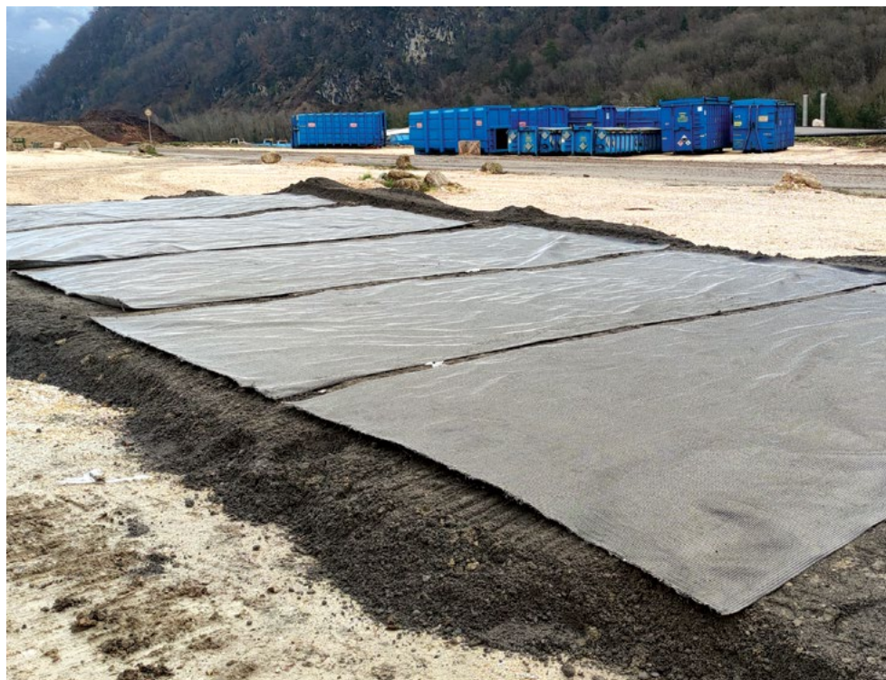
FIGURE 5 In situ tests with several types of soil over the geosynthetic
