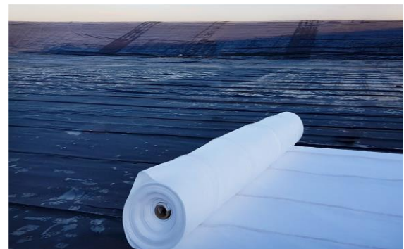
DRAINTUBE 400P FT1 D20 Conductive installation as leak detection layer between geomembranes. The geocomposite includes an electrically conductive layer on its upper part.
